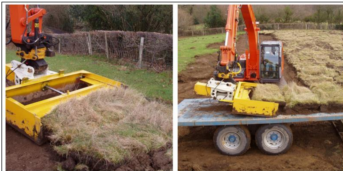
Figure 4-20: Example of modified turf excavator bucket for moving turves from trailer and placing them within temporary storage area/main receptor site (LEE, 2025)
